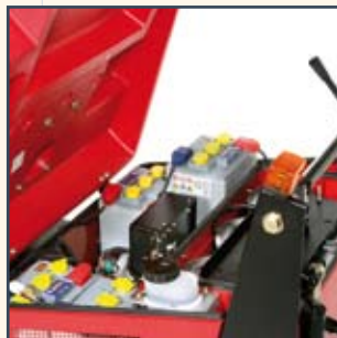
4 X 6V-180AH (5H) BATTERIES 4 BATTERIEN 6V - 180AH (5H) 4 6V-180AH (5H) ACCU'S
